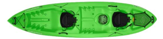
Lifetime has been informed of complaints of holes in the hull at the scuppers that could allow for water to enter the hull and the kayak itself to fill with water. The scuppers are hollows in the deck of the kayak that allow water to drain from the deck of the kayak.
