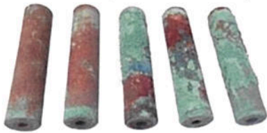
Before cleaning with wire brush (Natural “scaling” occurs during ionization)
