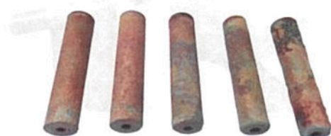
After cleaning with wire brush (You’ll see normal “pitting” after cleaning)
