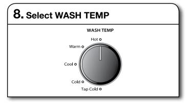
Once you select a cycle, select the wash temperature by turning the Wash Temp knob to the desired setting.
