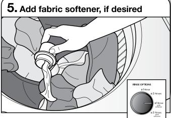
During the final rinse, wait until the washer has completed filling and press the START/Pause button to pause the washer. Lift the lid and add the measured, recommended amount of liquid fabric softener. Do not use more than the recommended amount. Close the lid and press the START/Pause button again to start the washer.
