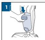
To release Dirty Water Tank, press down on recessed button on the top of the tank.
