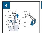
Remove strainer from Dirty Water Tank, then throw debris in trash.
