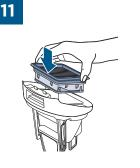
Place filter assembly back into the top of the Dirty Water Tank.
