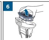
Remove the filter from the top of the Dirty Water Tank by pulling it up.
