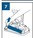
Pull Brush Roll out by grabbing the Brush Roll tab and pulling upward.
