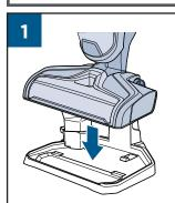
Lift and place your CrossWave® Cordless onto the 3-in-1 Docking Station to charge. 2
